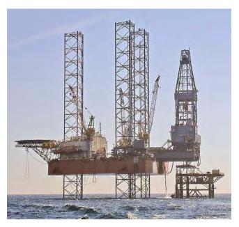
The rig is a self-propelled, semisubmersible unit which is able to drill to depth of 25,000 ft, in water depth of up to 1000 ft. Special design features enable normal drilling. The rig is able withstand galeforc for sustained periods when it is impossible to resupply due to weather conditions. The drilling rig has living quarters for 90 people.
