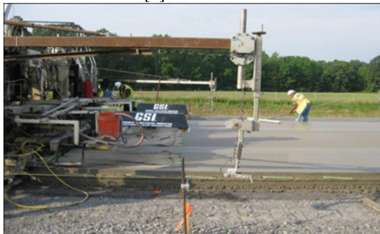
Figure 4. "GOMACO GSI" real-time profile measurement device installed on a cement mixer [6]
