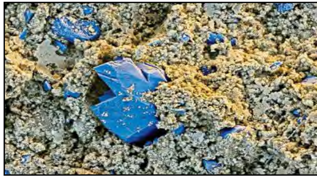
Fig.1 CRYSTALLIZING CONCRETE. This colorized scanning electron micrograph shows concrete (brown) crystallizing around X-Seed crystals (blue), 500 nm to 30 m across.
